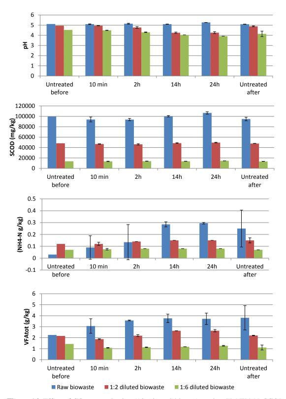
**Figure 14**. Effect of CO<sub>2</sub> pressurisation (10 min to 24 hours) on the pH, NH4-N, SCOD and VFAtot of biowaste as well as the effects of storage (4  $^{\circ}$ C, 4 days) on untreated samples. Averages with randomised standard deviations (RSD) are shown.
