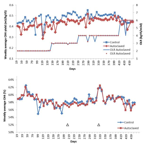
**Figure 5.** Weekly CH<sub>4</sub> yields and concentrations during days 19-388 in reactors R1 and R3 treating control and autoclaved food waste, respectively ( $\Delta$ =change of CH<sub>4</sub> concentration measurements).
