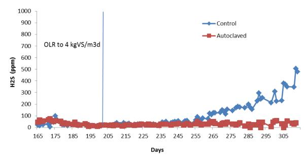
Figure 7. Hydrogen sulphide concentrations in control and autoclaved reactors during days 166-314.
