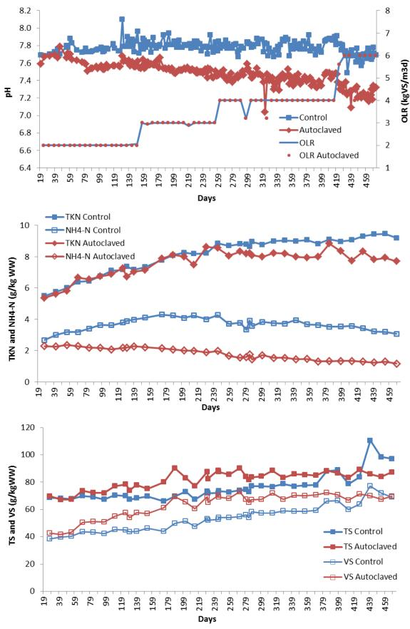
Figure 6. Reactor parameters from reactors R1 and R3 during days 19-470.
