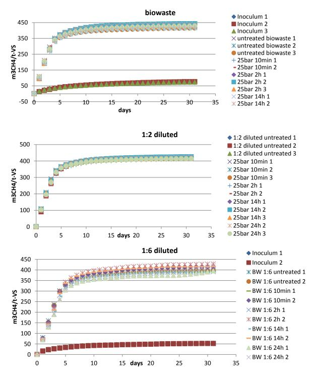
**Figure 15.** Specific methane productions of biowaste, 1:2 diluted biowaste and 1:6 diluted biowaste with different pressure treatment times
